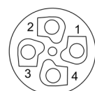
Screw terminal of the M12 female connector
