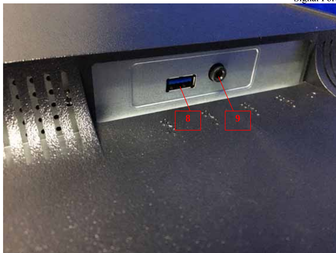
ESD Figure 3 Signal Port of the EUT
