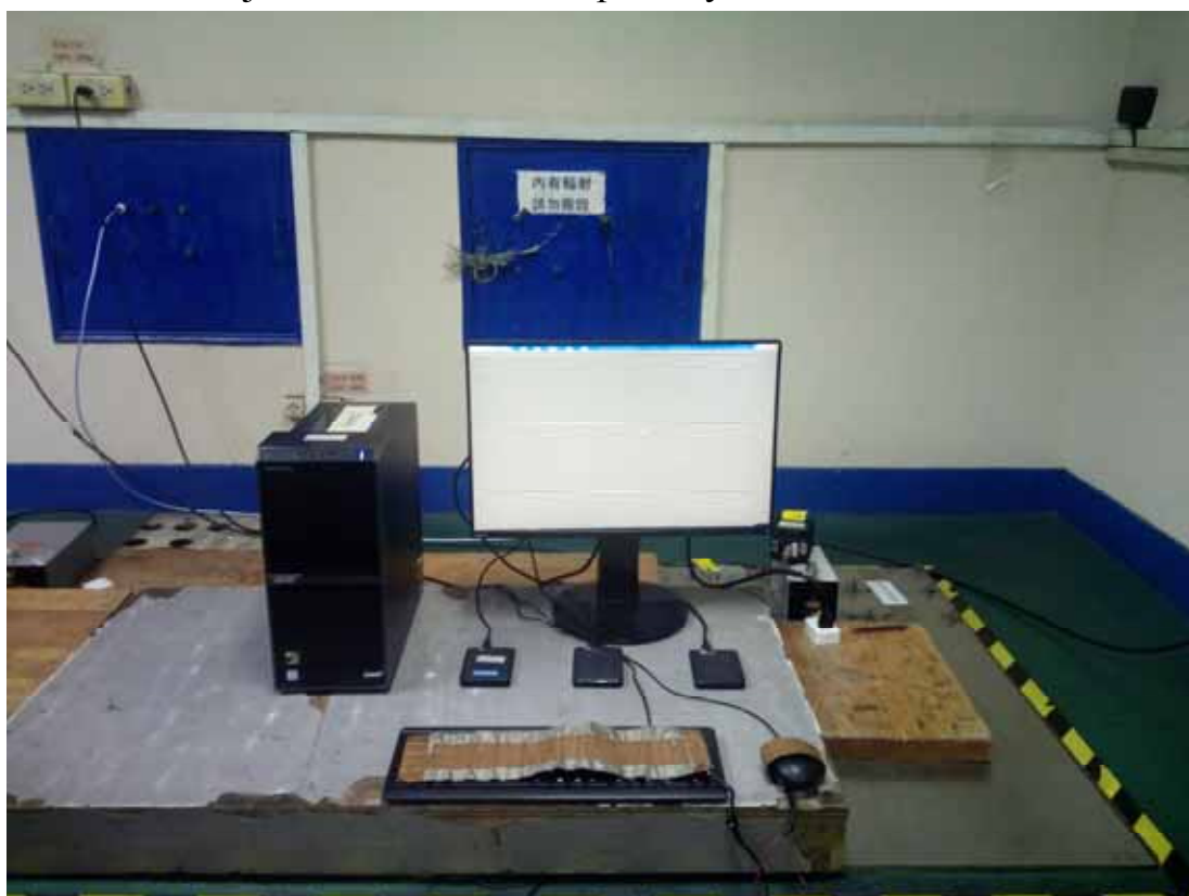
15.8. Photo of Injected Currents Susceptibility Test
